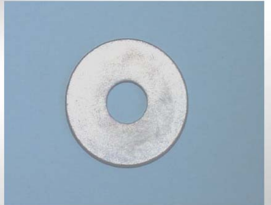
VACODYM 6xx: electrolytic Ni+Sn after 130°C/ 2.7 bar/ 100% humidity
